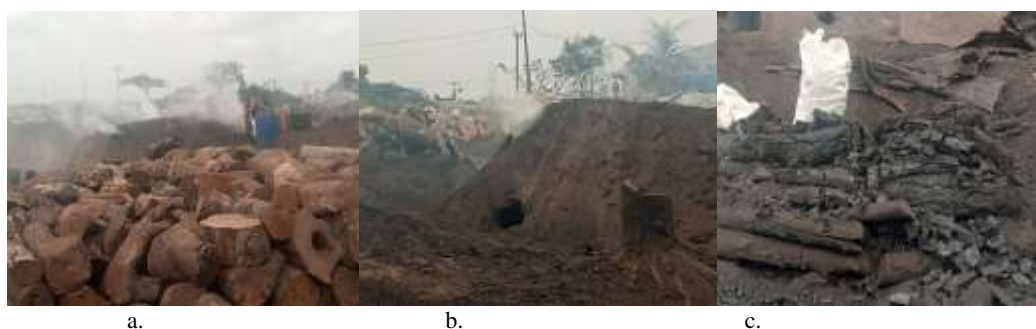
Plate 1 (a) starting materials (wood) for charcoal production (b) earth kiln for pyrolysis of wood (c) final product (charcoal)
